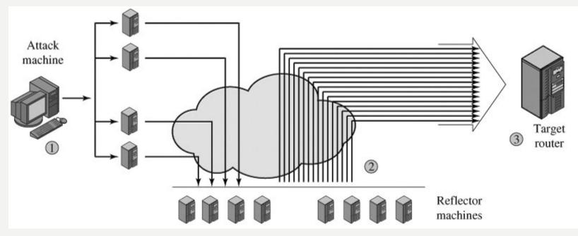
**ICMP** (Internet Control Message Protocol) is an errorreporting protocol network devices like routers use to generate error messages to the source IP address when network problems prevent delivery of IP packets موسيه آموزش عالى عسر دولتي عسراتناعي بفستر تيب
